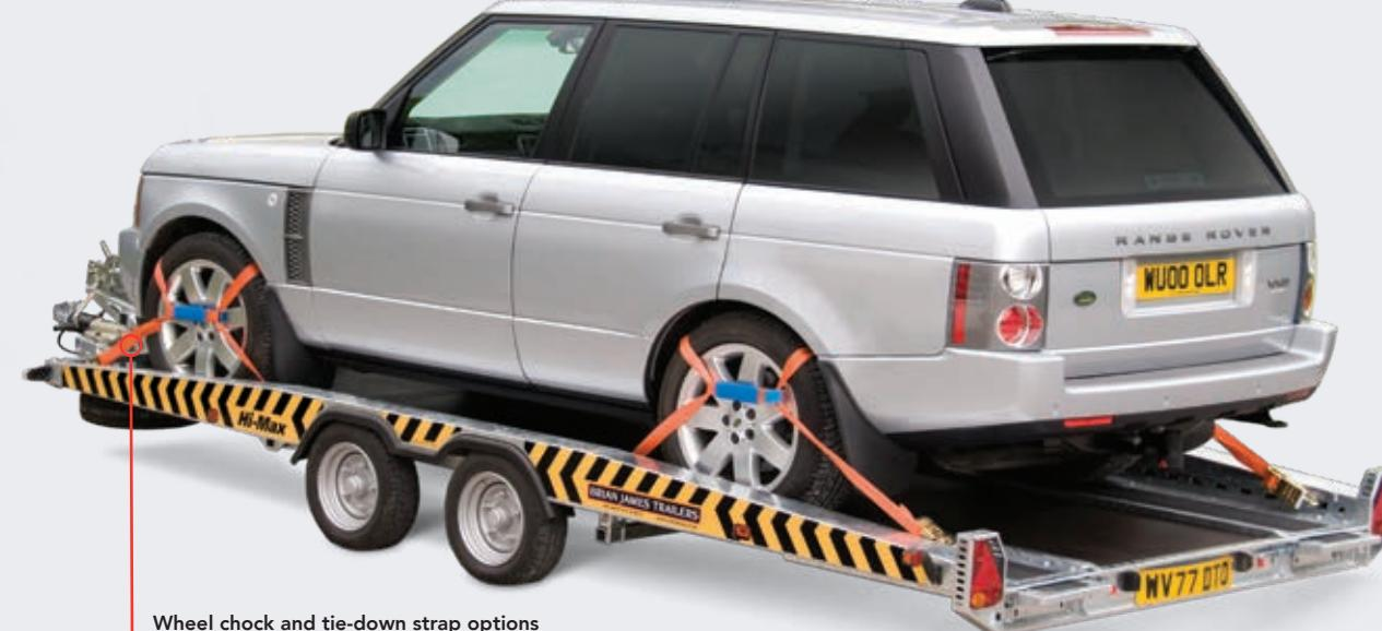
**Wheel chock and tie-down strap options** provides a flexible method of ensuring that the vehicle is always in the correct place.
